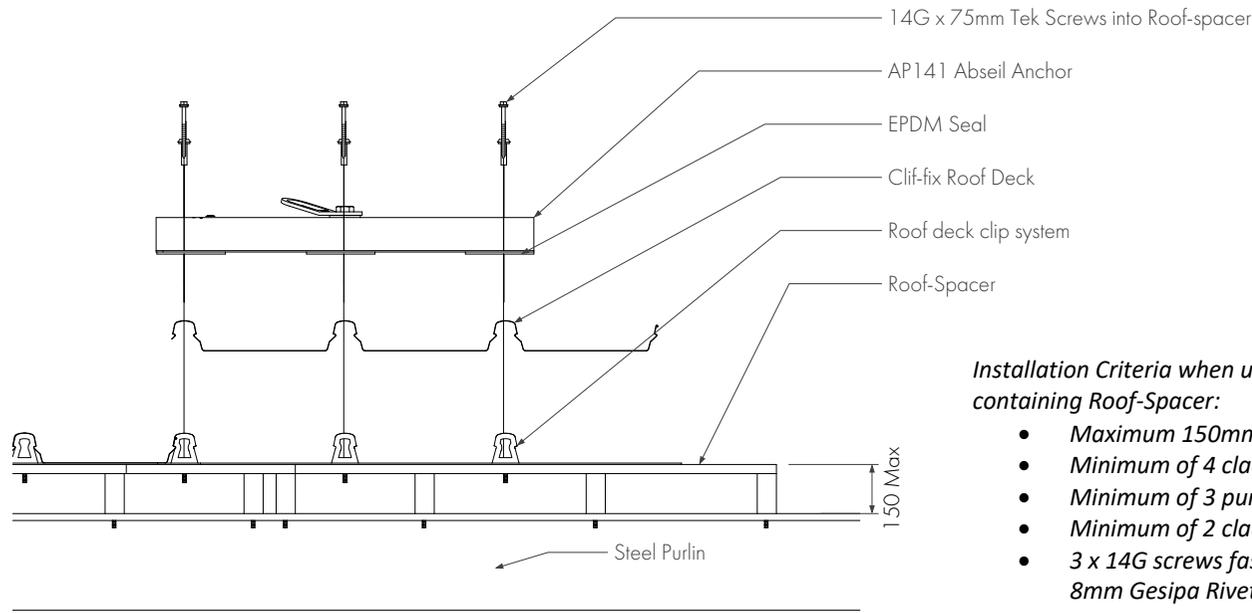
**Installation Criteria when using AP141 Abseil anchors on metal clad roofs containing Roof-Spacer:**
